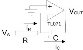
For the current through the cap , C=q/V so C=dq/dV and dq =idt so CdV= idt or i =CdV/dt then  $i_R=i_C$  since the – terminal is a virtual earth and  $i_C = -C dV_{OUT} dt = i_R = V_A/R dV_{OUT} = -V_A / RC dt$
