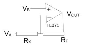
$$V_{OUT} = \left(\frac{R_F}{R_X} + 1\right) V_B - \left(\frac{R_F}{R_X}\right) V_A$$
