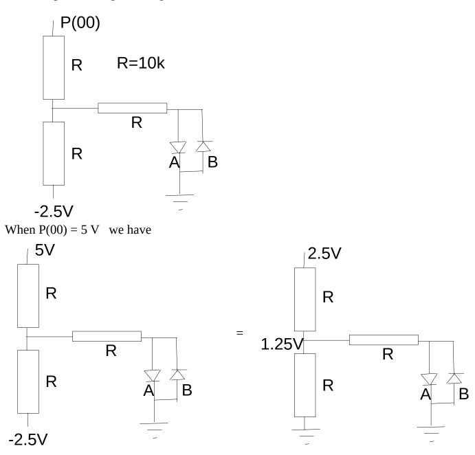
Here diode A is on and has an anode voltage of 0.8V which feeds the integrator.
