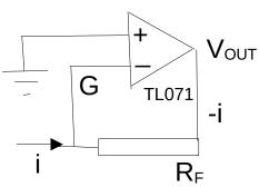
Point G is a virtual earth since the + input is grounded , so the output must supply current i = input current and  $V_{\rm OUT}$  =-  $R_{\rm F}i$
