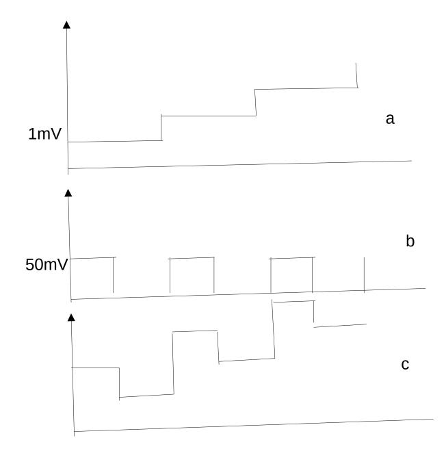
a can be produced by a clocked counter feeding a DAC
