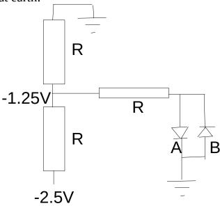
Now diode B is on with a cathode voltage of -0.8V which feeds the integrator. A relay (EDR201A0500) is used to short circuit the integrator capacitorand switch the integrator capacitor off. The  $27\Omega$  resistor is to prevent a spark when discharging the capacitor. To swith the integrator on the relay must be open P(01) must be high. AI0 captures the voltage of the we while AI1 captures the current related voltage. The voltammeter is switched on by closing the relay.
