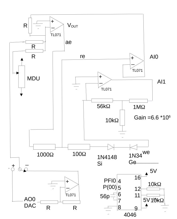
A digital I/O P(00) is used to switch the 4046 clock on. The output of the 4046 on pin 4 goes to the PFIO input on the USB6008 and now we can time anything to an accuracy of 1.2uS.
